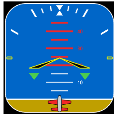
Fig. 6 Envelope protection warning (pitch down).
