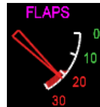
Fig. 7 Envelope protection warning (raise flaps).
