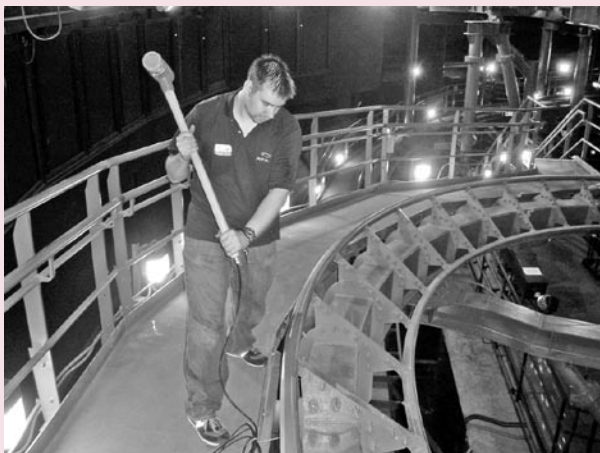
Jeff Kowtko performs a vibration test on "Space Mountain" at Disneyland in Anaheim, California.
