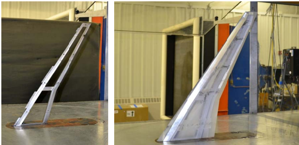
Figure 1: The steel frame and complete model used in wind tunnel testing in the University of Illinois 3'x4' tunnel. Only the complete model on the right is used in testing.
